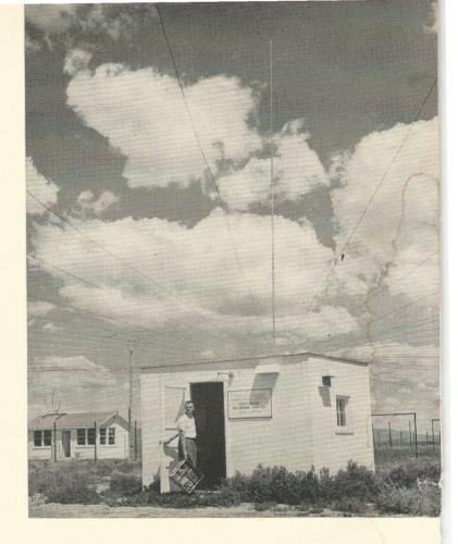
second. In addition, some have been modified to record also the average noise voltage and the average of the logarithm of the noise voltage. It has been shown that these three statistical characteristics of the noise provide a reasonably comprehensive picture of the physical nature of its amplitude distribution.
