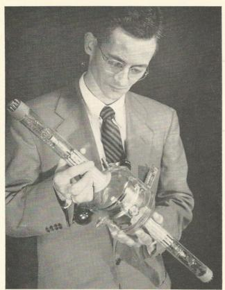
A Naval Research Laboratory scientist, F. H. Harris, holds a "regenerated electrical output storage tube" (REO to those who work with it). The tube differs from other types in that its "reading time" can be extended to hours or even days. It is capable of capturing a single frame of a television picture, recording maps, mathematical function curves, and performing many tasks where a "memory" is needed. Its ability to hold an image is expected to have military and industrial values.
