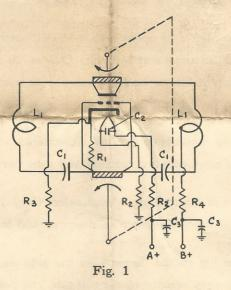
Circuit diagram of the 140-450 Mc. oscillator. The oscillator tube is a 6F4, drawn here in unconventional fashion to show how the tube elements are tied in with circuit construction.
