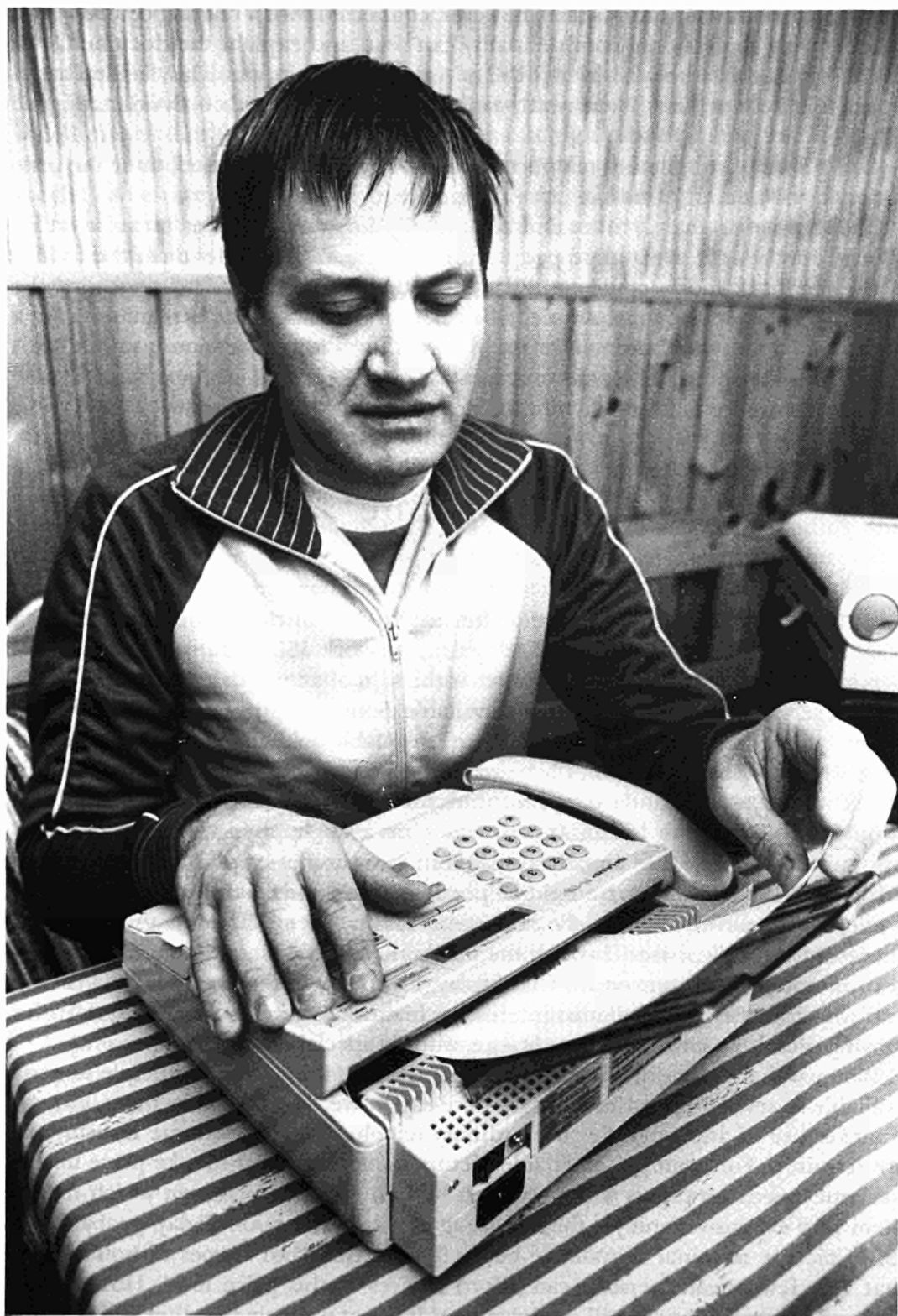
Figure 33.4 A telefax machine is used as input device for a blind person's remote reading service.
