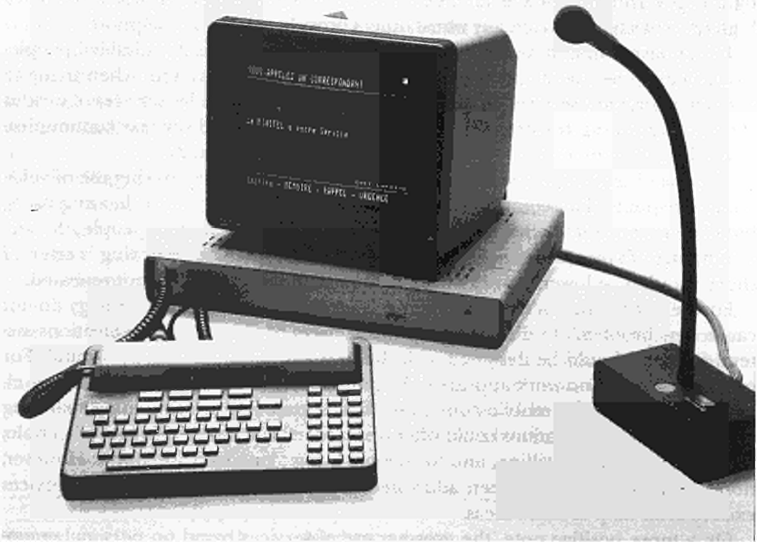
Figure 14.3 Covotel from CNET. This combined telephone and Minitel terminal is operated by voice. The telephone number can be dialled one by one or by choosing from a list of 60 numbers. Minitel commands are also available.
