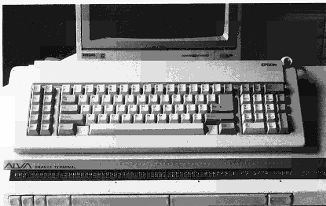
Figure 43.4 A one line Braille display placed below a computer keyboard.
