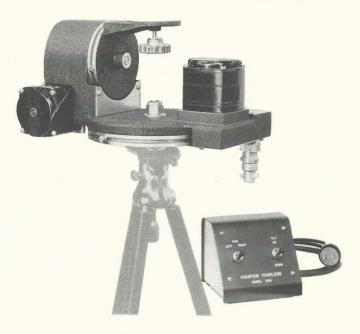
or table or mounted on a panel (on special order) for relay rack installation. The connecting cable (not furnished) may be 20 gauge, 5 conductor Alpha 1247 or equal. Cable connectors are supplied. For distances up to 500 ft., 22 gauge is satisfactory; up to 1000 ft., 20 gauge; up to 2000 ft., 18 gauge.
