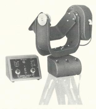
A ten wire cable (not furnished, connectors only furnished), is required between the control unit and the head. Specified sizes for various distances are: 100 ft.—24 gauge. 200 ft.—22 gauge. 500 ft.—18 gauge. 1000 ft.—14 gauge. 2000 ft.—12 gauge.
