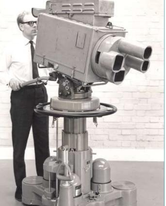
▲ Vinten 419 pedestal with Mk III pan and tilt head supporting a CPS Emitron camera. This is the 419 in its classic form after a ringsteer had been added
