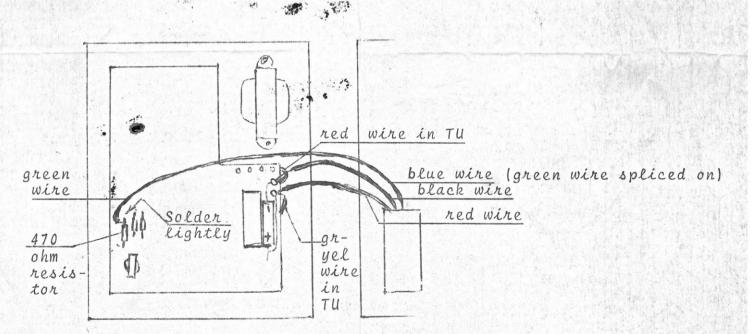
Solder the end of the green wire <u>lightly</u> to the (upper) wire leading out of the 470-ohm resistor. Use a small pencil soldering iron, of about 30-watt size, and do not overheat the connection, as it is connected to a printed circuit foil below. A tab of solder should hold the wire nicely without falling off.
